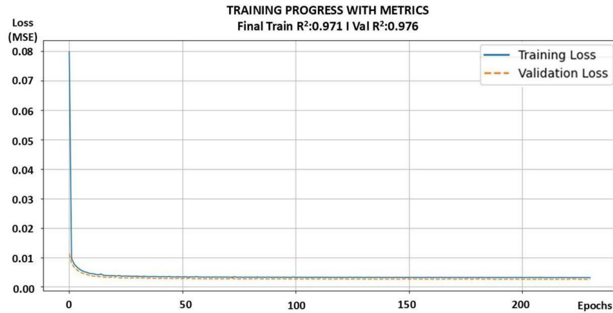
Figure 12: Performance metrics for the CNN-based 3D gravity inversion model. The training set yielded an MSE of 3.12 \times 10^{-3} , RMSE of 0.0558, R^2 of 0.9708, and accuracy of 96.20%. The validation set demonstrated comparable performance, yielding a low mean squared error (MSE) of 2.56 \times 10^{-3} , RMSE of 0.0506, R^2 of 0.9756, and accuracy of 95.960%, indicating high predictive accuracy and generalization.
